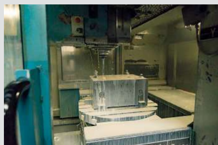
Fuel injection pump block (2-stroke engine) during drilling process
